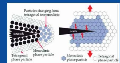
Figure 12: M Phase Transformation Toughening Schematic
