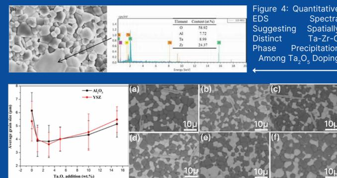
Figure 5: Resultant  $Ta_2O_5$  Addition Effect on YSZ and  $Al_2O_3$  Average Grain Size (left) and Corresponding YSZ Micrographs from Low (a) to High (f)  $Ta_2O_5$  Addition (right) Among 0, 1, 3, 5, 10, and 15wt%  $Ta_2O_5$  Dopant Concentrations
