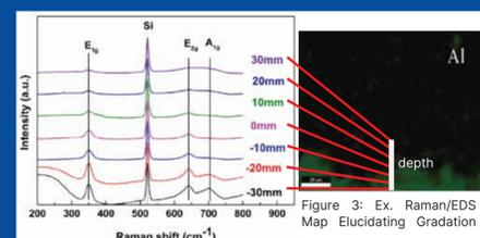
Raman and EDS determine Ta's penetration depth and gradation profile in Ta-Doped YSZ cross-section through EDS corroborated Peak Transformation Analysis
