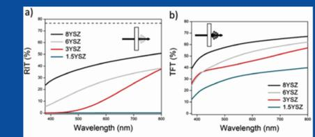
Figure 11: Real In Line (RIT) and Total Forward Transmission (TFT) of 1.5mol% - 8mol% Yttria Concentrations in YSZ, Revealing Translucency Increase
