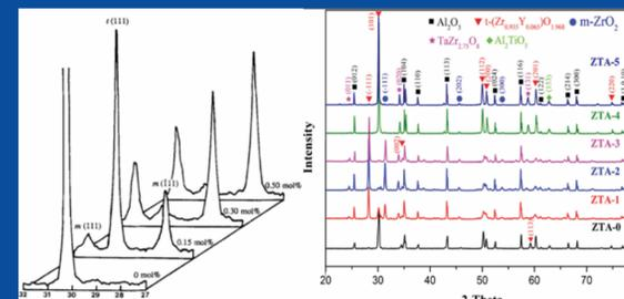
Figure 7: Increasing  $Ta_2O_5$  concentration's inverse effect on tetragonal YSZ phase stability (left), and significant  $TaZr_{2.75}O_8$  phase precipitation (right) for YSZ toughened alumina (ZTA) of increasing (ZTA-0 to 5) Ta concentration
