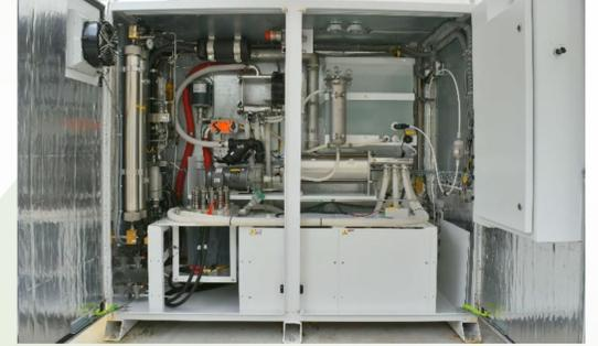
Photograph of the 60kW PEM electrolyzer used in the first U.S. pilot of P2G
